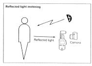
exposure which will reproduce the metered area as a tone with 18% reflectance (zone 5) regardless of its true shade.
